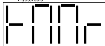
Fig. D18 -- Programming Mode Timer or Timer Mode Active
