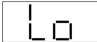
Fig. D46 – Programming Condition ALARM Lo setting
