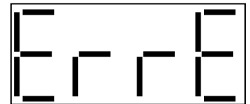
Fig. D65 – Error Condition Memory Error
