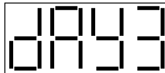
Fig. D51 – FAILURE Condition CLOCK Circuitry failure
