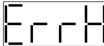
Fig. D64 – Error Condition Hardware Error
